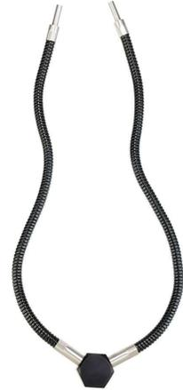
**FOI-2** - A single strand semi-rigid (will hold it's shape) light guide, .500" outside diameter Metal Sheathing, .250" fibre optic light guides. This unit is 48" long and can be mounted on a machine tool for extra illumination.
